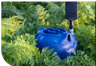
CROPX VERTEX 4 (V4) All-in-one smart soil sensor
