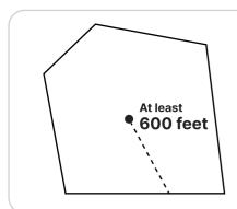
For in field installations with 600 feet (183 meters) or more to the planted field edge, please use the following instructions for mounting the sensor onto the center pivot system.
