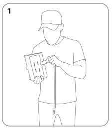
Slide the hose clamps through the slots in the back of the telemetry unit.
