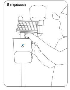
Attach the Rain gauge to the lightning pole using the hose clamps and the cable to the "Pulse" input of the telemetry unit (use A first)
