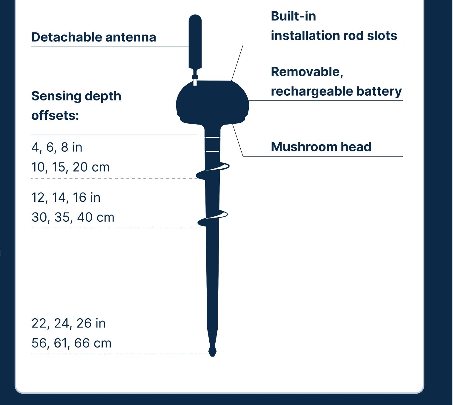
Virtual sensing - calculating moisture every 4" from 8"to 26", or every 10 cm from 20 cm to 66 cm
