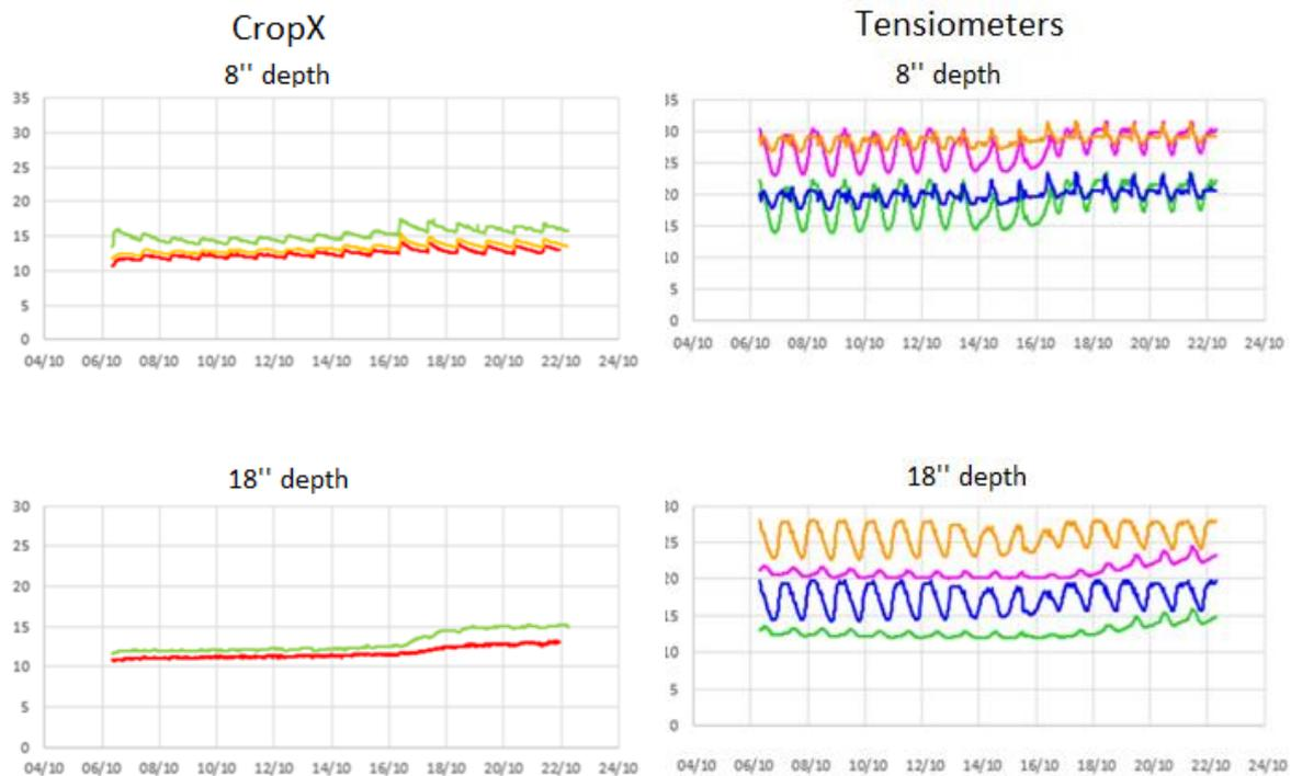
The larger spikes in the tensiometer graphs are a result of preferential flow along the tensiometer tube. This shows that the unique geometry of the CropX probes minimize result in readings that better reflect the actual soil moisture.
