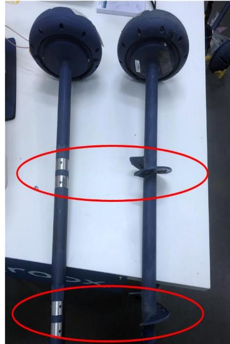
Probes without the spirals showed a more significant water movement and responded significantly earlier (45-75 minutes) than probes with spirals. Absolute reading of sensors on spirals are higher due to higher soil density in the undisturbed soil.
