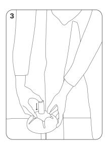
Mount the sensor head adapter in the grooves on top of the sensor head
