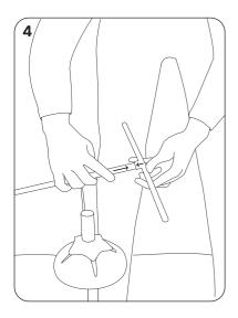
Mount the handle on the sensor head adapter and tighten it.
