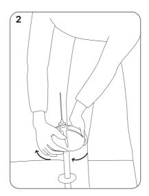
Insert the sensor into the hole and screw it gently, until it stands firmly in the ground. Do not apply downward force.
