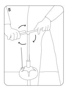
Screw the sensor almost all the way down using the handle, leaving a 1finger gap between the ground level and the bottom of the sensor head.
