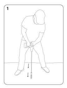
Drill a vertical hole in the soil using your drill and the provided drill bit. If necessary, drill and retract several times until the bit reaches the full depth
