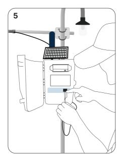
Connect the thermocouple connector to the slot provided. (See the wiring scheme below)
