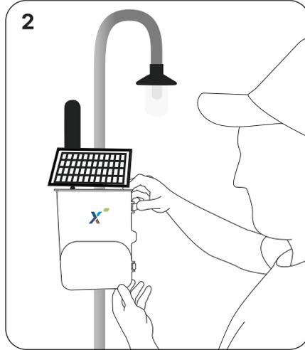
Securely install the telemetry device to the light pole located on your pivot using the hose clamps or zip ties from the previous step.
