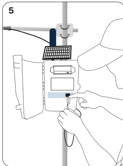
Connect the thermocouple connector to the slot provided. (See the wiring scheme below)
